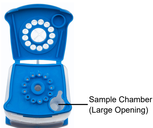
Figure 5. Xpert Xpress CoV-2/Flu/RSV plus Cartridge (Top View)
