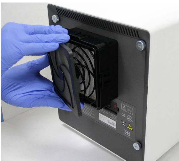
Figure 9-25. Removing the Prefilter Retainer
