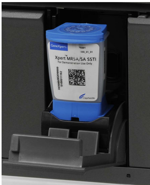
Figure 5-33. GeneXpert Cartridge, Positioned at the Heel of the Module Bay Floor
