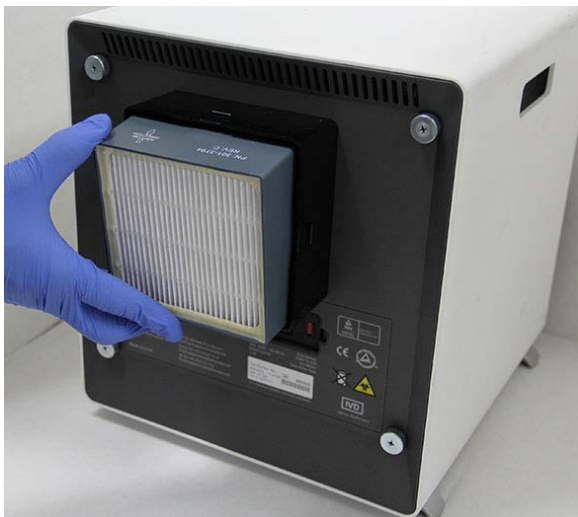
Figure 9-29. Replacing the HE Filter
