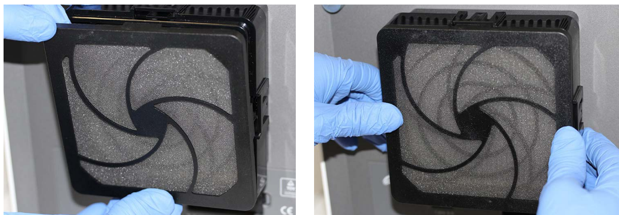
Figure 9-31. Replacing the Prefilter and the Prefilter Retainer
