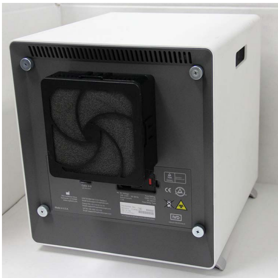
Figure 9-24. GX-IV Instrument Positioned for Access to Filter
