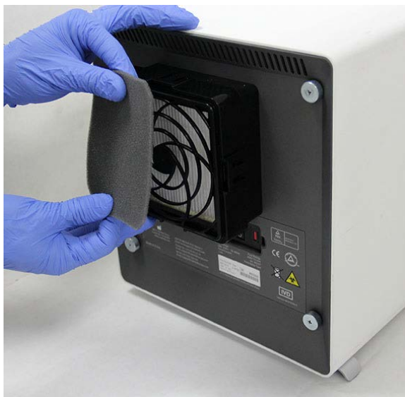
Figure 9-26. Removing the Prefilter
