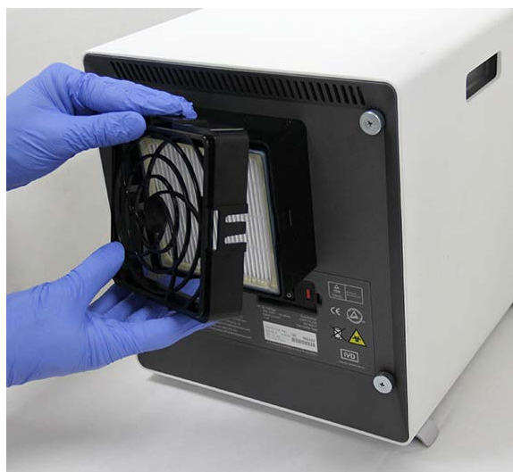
Figure 9-27. Removing the HE Filter Retainer
