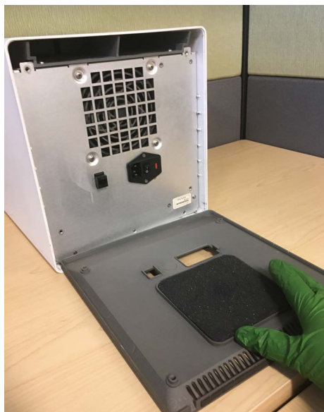
Figure 9-16. Replacing Foam Filter in Older GX-IV
