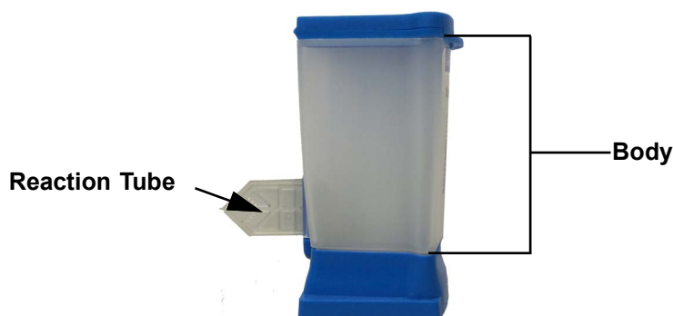
Figure 5-31. Cartridge Showing Body and Reaction Tube
