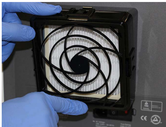
Figure 9-30. Replacing the HE Filter Retainer
